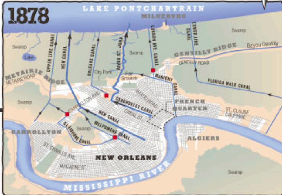
DRAINING THE SWAMP - City officials get serious about storm drainage. A series of smaller canals are created to feed into three major ones: London Avenue, Orleans Avenue and what would later be called 17th Street. One official urges that pumping stations be placed at the lake to prevent storm surge from flowing into the city. But no one listens. Meanwhile, city officials turn to the canals for a new mission. With the high ground all developed, they see the swamp between settled areas and Lake Pontchartrain as a new source of land.
