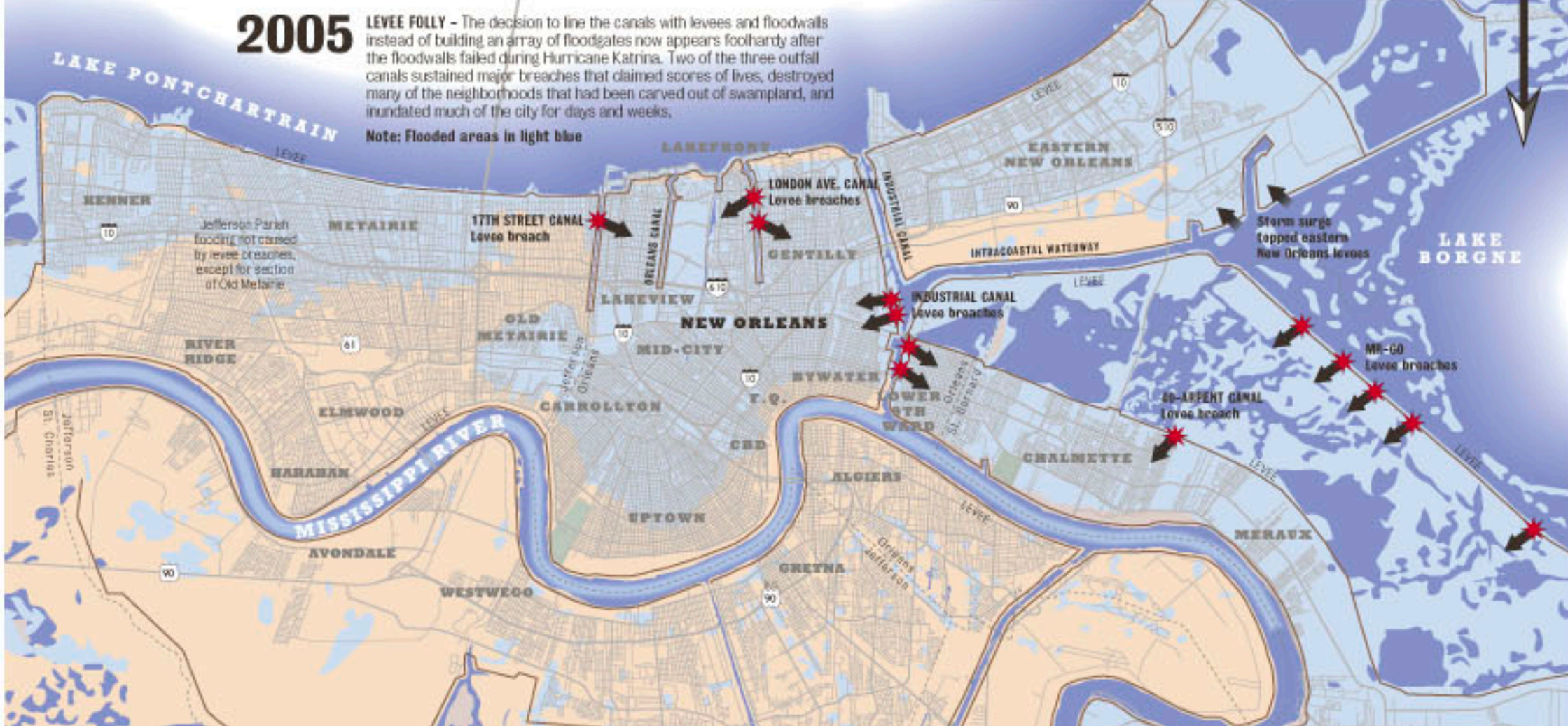
TODAY'S SYSTEM - The modern system now includes 1,258 miles of drainage pipes, 170 miles of canals and more than 20 pumping stations. The three large outfall canals remain the major conduits for removing water. When the Army Corps of Engineers suggests placing floodgates at the end of those canals, the city — worried about the impact on the system's ability to pump out rainwater — objects. The city prevails, and a system of canal levees and floodwalls are built.
