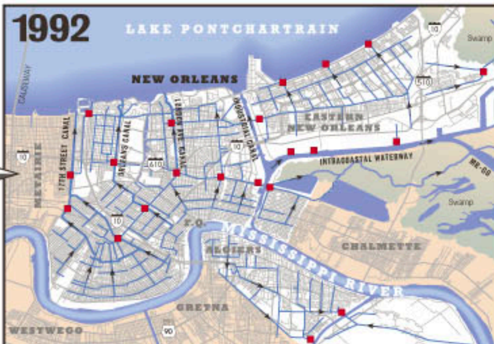
TODAY'S SYSTEM - The modern system now includes 1,258 miles of drainage pipes, 170 miles of canals and more than 20 pumping stations. The three large outfall canals remain the major conduits for removing water. When the Army Corps of Engineers suggests placing floodgates at the end of those canals, the city — worried about the impact on the system's ability to pump out rainwater — objects. The city prevails, and a system of canal levees and floodwalls are built.
