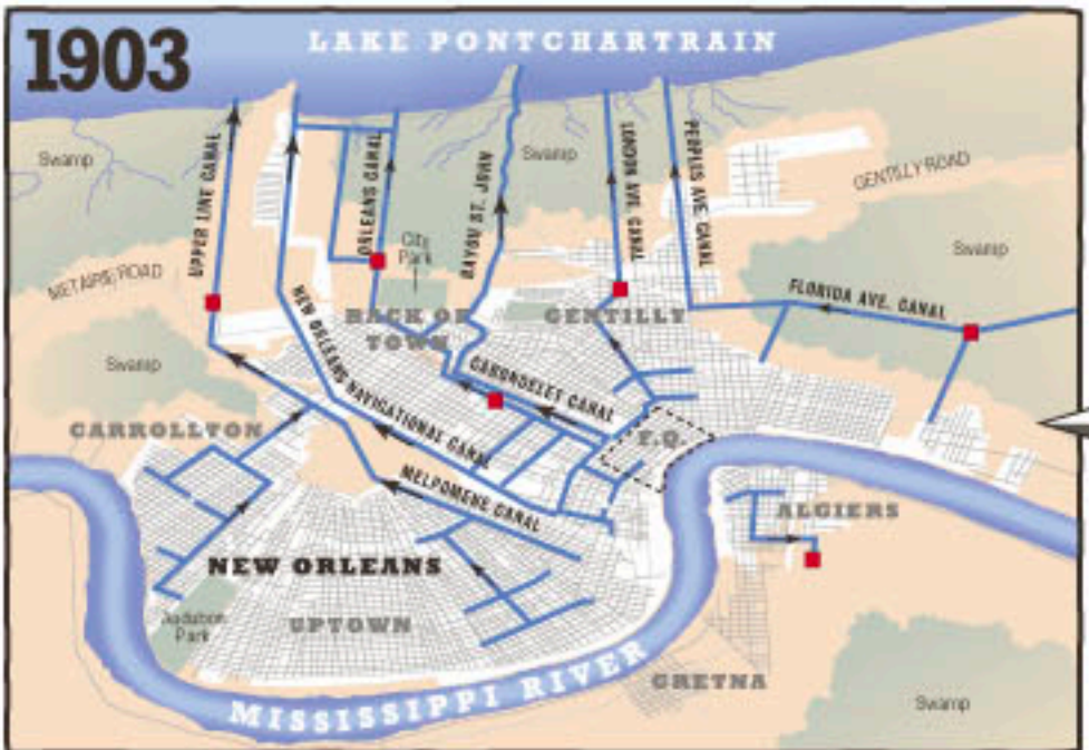
MODERN DRAINAGE - At the turn of the century, the city embarks on a 15-year, $27 million project that would create the world's most advanced drainage system. It would include 70 miles of canals and an innovative series of locally designed screw pumps. Elements of the system are still in use today.
